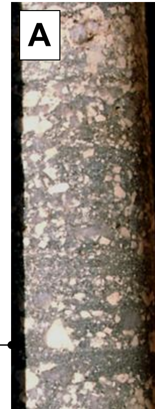
A. Lower arkose, coarse feldspars with shear zones evident within samples.
