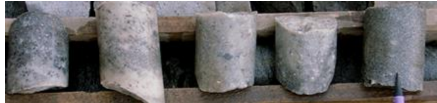
D. Sericite quartz alteration of Upper Orebody in NE511
