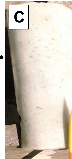
C. Carrollite bearing upper arkose with variable amounts of dolomite
